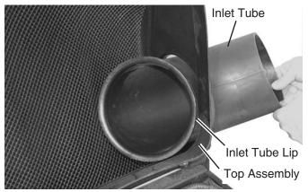
**C.** After the inlet tube is in place attach the 6" hose to the inlet tube and the boot assembly. Use the two large hose clamps supplied in the bag of hardware. For best collection results, trim hose so there is no more than 2 inches excess hose with mower deck in the lowest position. Refer to (Figure 14).
